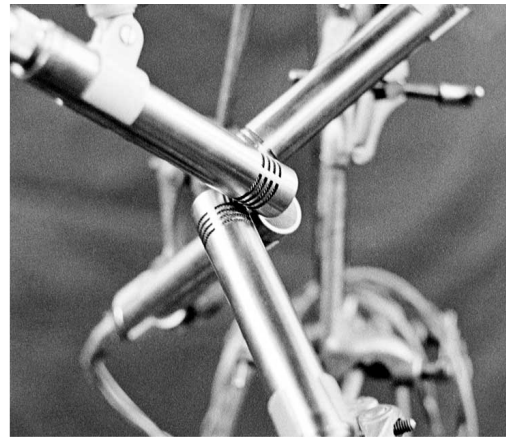
Fig. 3 Experimental tetraphonic array using Calrec capacitor microphones
